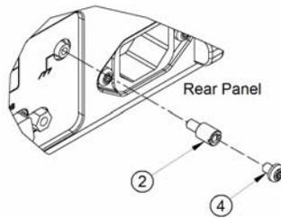
3. Use the flat-blade screwdriver to turn the extender approximately  $\frac{1}{4}$  turn past finger tight, or use a calibrated torque tool with a flat-blade screwdriver bit to torque the extender to 10 in-lb (11.5 kilogram-centimeter).
